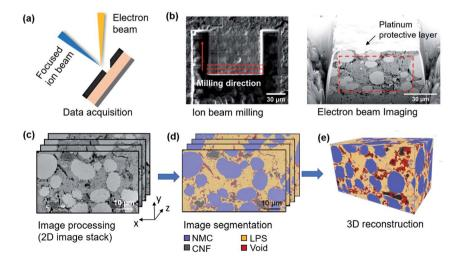
Fig. 2 Workflow for FIB-SEM tomography. (a) Schematic illustration of data acquisition set-up in FIB-SEM. (b) Ion-beam milling and BSE electron beam imaging were performed iteratively during serial sectioning. (c) 2D image stack obtained after image processing. (d) Corresponding four-phase segmentation results and (e) reconstructed 3D volume of the cathode composite (the final 3D volumes were slightly different for the three samples but were all  $\sim 60 \times 40 \times 30 \ \mu m^3$ ).
