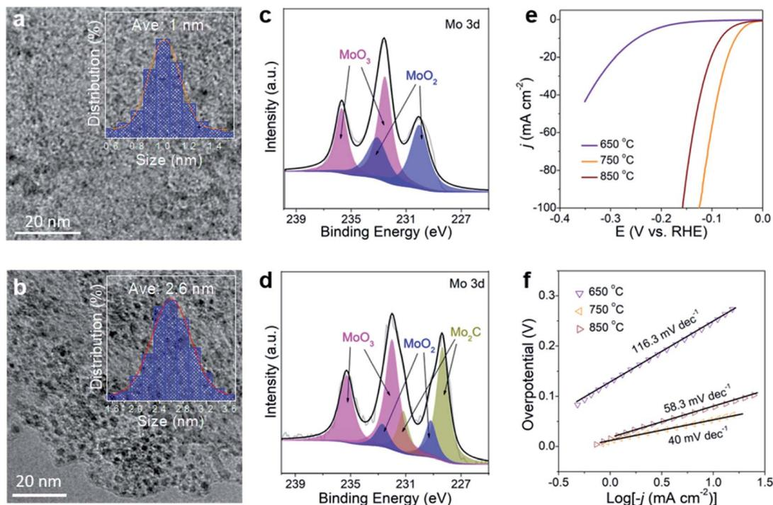
Fig. 5 TEM images of (a) M-650 and (b) M-850. The inset gives the size distributions of nanoparticles in the samples. High-resolution XPS Mo 3d spectra of (c) M-650 and (d) M-850. Polarization curves (e) and Tafel plots (f) of M-650, M-750, and M-850.
