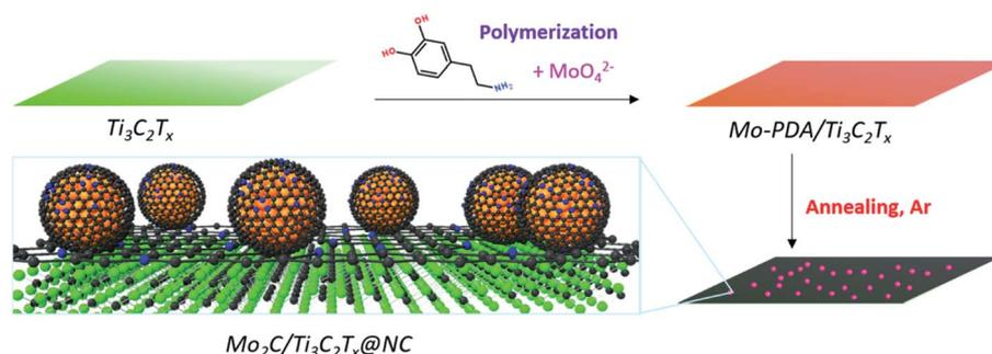
Fig. 1 Synthetic illustration of the preparation of Mo<sub>2</sub>C/Ti<sub>3</sub>C<sub>2</sub>T<sub>x</sub>@NC.
