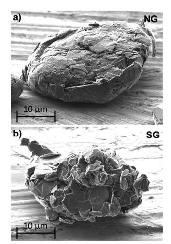
Fig. 10 Comparison of SEM micrographs of sphere-shaped natural graphite (NG; after several processing steps) and synthetic graphite (SG).
