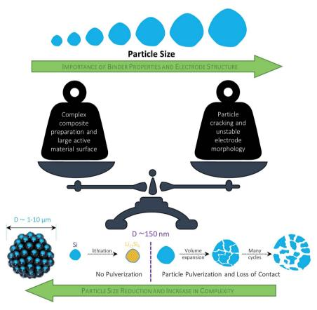
Fig. 15 Schematic summary of the trade-off between the advantages of a reduced particle size for the silicon active material and the accompanying challenges with respect to particle pulverization, active material surface, electrolyte decomposition at the electrode/electrolyte interface, mechanical properties of the electrode, and packing density (figure inspired by and redrawn from ref. 338 and 339).
