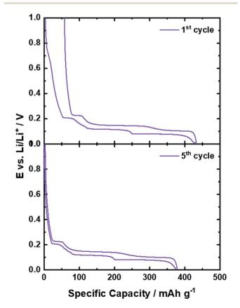
Fig. 5 Comparison of the potential profile of graphite half-cells for the  $1^{\rm st}$  (upper panel) and  $5^{\rm th}$  (lower panel) dis-/charge cycle.
