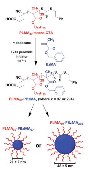
Scheme 1 A PLMA $_{39}$  precursor block is chain-extended with BzMA monomer in n-dodecane via RAFT-mediated PISA to form sterically-stabilized spherical nanoparticles. SAXS analysis (see Fig. S3, Tables S2 and S3 in the ESI†) indicated that final PBzMA DPs of 97 and 294 produced mean core diameters of 21  $\pm$  2 nm and 48  $\pm$  5 nm, respectively.
