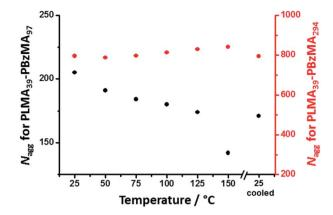
Fig. 2 Temperature dependence for the mean aggregation number (N<sub>agg</sub>) determined by SAXS analysis of 1.0% w/w dispersions of (black) PLMA<sub>39</sub>-PBzMA<sub>97</sub> and (red) PLMA<sub>39</sub>-PBzMA<sub>294</sub> spheres at various temperatures. The former spheres exhibit a significant reduction in  $N_{\text{agg}}$  on heating, while the latter exhibit minimal change in aggregation number.
