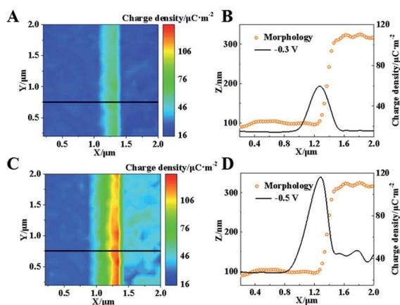
Fig. 4 (A) Charge density of the Pt-graphite interface at a voltage of  $-0.3\text{ V}$ . (B) Morphology and charge density along the black line in (A). (C) Charge density of the Pt-graphite step at a voltage of  $-0.5\text{ V}$ . (D) Morphology and charge density along the black line in (C).
