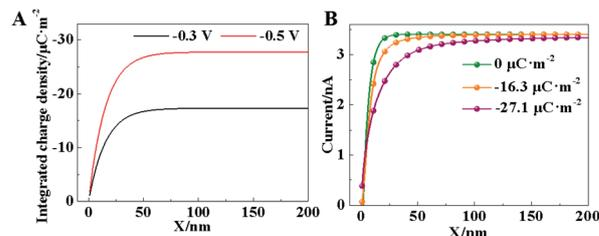
Fig. 2 (A) Theoretical curves of integral charge density within the diffuse layer with the applied voltages of  $-0.3$  and  $-0.5$  V. (B) Theoretical approach curves of the SICM current with different charge densities within the diffuse layer.
