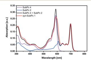
Fig. 3 Steady-state absorption spectra of  $syn\text{-SubPc}~\mathbf{1}~(1.5\times10^{-6}~\text{M}),$  dimer-SubPc  $\mathbf{2}~(1.5\times10^{-6}~\text{M})$  and monomer-SubPc  $\mathbf{4}~(3.0\times10^{-6}~\text{M})$  in toluene. The black spectrum relates to that of a 1:2 mixture of  $\mathbf{2}$  and  $\mathbf{4}$ .
