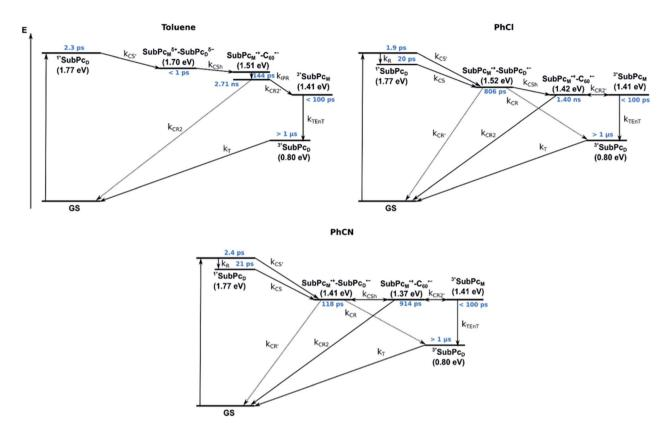
Fig. 13 Energy diagrams of syn-SubPc  $1-C_{60}$  in toluene, PhCl, and PhCN illustrating the excited state deactivation after 656 nm laser excitation at room temperature. Lifetimes were obtained by global analysis of the transient absorption data. Solid lines represent major pathways and dotted lines, minor ones.
