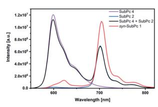
Fig. 4 Steady-state fluorescence spectra of syn-SubPc 1 (1.5  $\times$  10<sup>-6</sup> M), dimer-SubPc 2 (1.5  $\times$  10<sup>-6</sup> M) and monomer-SubPc 4 (3.0  $\times$  10<sup>-6</sup> M) in toluene. The black spectrum relates to that of a 1 : 2 mixture of 2 and 4.  $\lambda_{\rm ex}=530$  nm.
