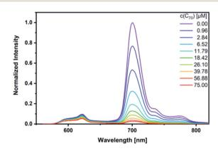
Fig. 6 Steady-state fluorescence spectra of syn-SubPc 1 (1.5  $\times$  10<sup>-6</sup> M) after 440 nm excitation in toluene with increasing amount of C<sub>70</sub> (0–75  $\mu$ M).
