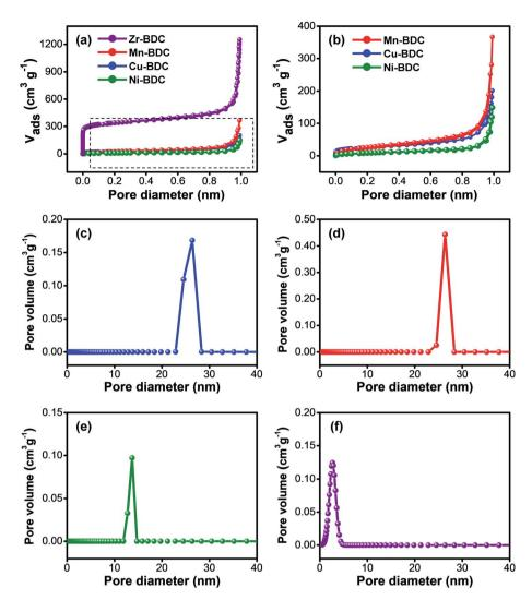
Fig. 4 (a) Nitrogen ( $N_2$ ) sorption isotherms of all prepared M-BDC products. (b) Enlarged  $N_2$  sorption isotherms of the as-synthesized Mn-BDC, Cu-BDC, and Ni-BDC samples. NLDFT pore size distribution plots of (c) Cu-BDC, (d) Mn-BDC, (e) Ni-BDC, and (f) Zr-BDC.
