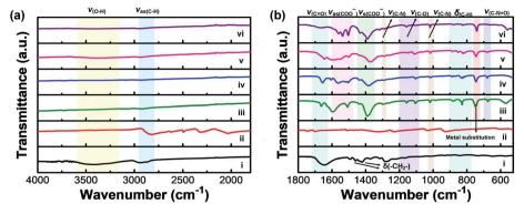
Fig. 2 FTIR spectra of (i) pure PVP, (ii) H<sub>2</sub>BDC ligand and the as-prepared M-BDC products: (iii) Cu-BDC, (iv) Mn-BDC, (v) Ni-BDC, and (vi) Zr-BDC in the wavenumber regions of (a)  $4000-1800 \text{ cm}^{-1}$  and (b)  $1800-525 \text{ cm}^{-1}$
