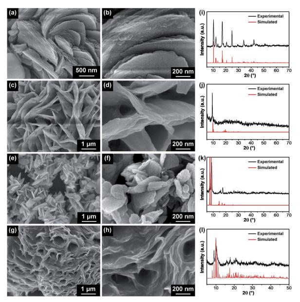
Fig. 1 Low- and high-magnification SEM images of M-BDC products obtained with the optimized mass ratios of metal precursor to PVP: (a and b) Cu-BDC (1:3), (c and d) Mn-BDC (1:5), (e and f) Zr-BDC (1:5) and (q and h) Ni-BDC (1:3). Experimental, simulated and reference PXRD patterns for Cu-BDC(i), Mn-BDC (j), and Zr-BDC (k). (l) Experimental and simulated PXRD patterns for Ni-BDC.
