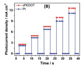
Fig. 3 (A)  $J_{sc}$  values plotted as a function of different light intensities for ASCs assembled with different cathodes. (B) Transient photocurrent measurements under different light intensities for the two cells in panel A.
