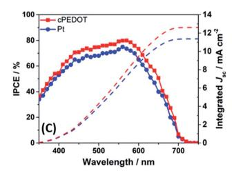
Fig. 2 (A) Photocurrent density vs. photovoltage curves for the three best ASCs fabricated with different cathodes and measured under 1 sun irradiation (AM1.5G). (B) Statistics of 30 devices collected over 3 different batches: PCE values are shown for ASCs assembled with different cathodes. (C) IPCE and integrated  $J_{\rm sc}$  for the same cPEDOT-and Pt-based devices shown in panel A.
