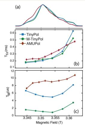
Fig. 5 (Top) W-band (~94 GHz) echo-detected EPR spectra of 100  $\mu M$  TinyPol, M-TinyPol and AMUPol solutions in d $_8$ -glycerol/D $_2O/H_2O$  60/30/10 (v/v/v) recorded at 100 K. (Middle) Electron spin lattice relaxation time ( $T_{1e}$ ) and (bottom) electron phase memory time ( $T_{m}$ ) measured at various position of the magnetic field. See ESI for Experimental details.†
