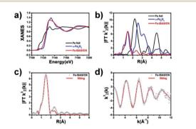
Fig. 2 (a) XANES spectra of Fe-ISAS/CN, Fe foil and  $\alpha$ -Fe<sub>2</sub>O<sub>3</sub> at the Fe K-edge. (b) Fourier transform (FT) spectra at the Fe K edge of Fe-ISAS/CN, Fe foil and  $\alpha$ -Fe<sub>2</sub>O<sub>3</sub>. (c and d) The fitting results of the EXAFS spectra of Fe-ISAS/CN in *R* space and *k* space, respectively.
