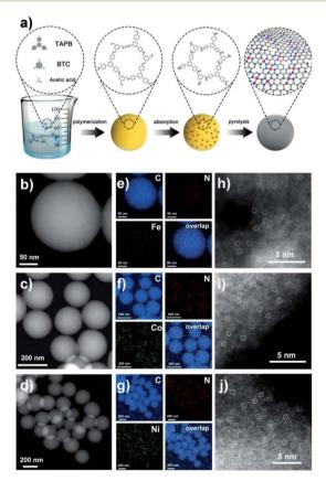
Fig. 1 (a) Schematic illustration of the synthetic process of metal ISASs anchored on COF-derived N-doped carbon nanospheres. (b)-(d) HAADF-STEM images of Fe-ISAS/CN, Co-ISAS/CN and Ni-ISAS/CN, respectively. (e)-(g) Corresponding energy dispersive X-ray spectroscopy elemental mapping results of Fe-ISAS/CN, Co-ISAS/CN and Ni-ISAS/CN, respectively. (h)-(j) AC-STEM images of Fe-ISAS/CN, Co-ISAS/CN and Ni-ISAS/CN, respectively; metal ISASs are highlighted with white circles for better observation.
