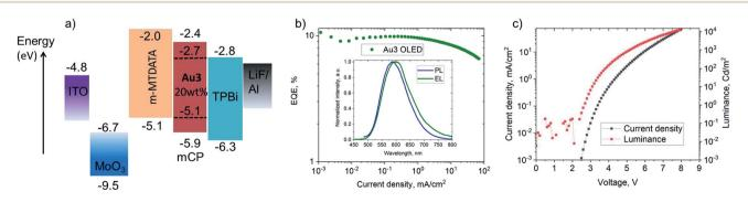
(a) Vapour-deposited OLED device architecture based on Au3; (b) external quantum efficiencies vs. current density of champion OLEDs with inset showing the electroluminescence (EL) and PL spectra; (c) current density/luminance vs. voltage curve of champion OLEDs.
