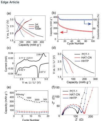
Fig. 4 (a) Galvanostatic charge–discharge profiles of PCT-1 at 500 mA  $\rm g^{-1}$ . (b) Capacity and coulombic efficiency of the battery. (c) CV profile of PCT-1 for the first cycle. (d) Galvanostatic charge–discharge profiles of PCT-1, HAT-CN, and HHTP at 500 mA  $\rm g^{-1}$  for the second cycle. (e) Rate performance of PCT-1 (black), HAT-CN (red), and HHTP (blue) at 500–2000 mA  $\rm g^{-1}$ . (f) EIS profiles of PCT-1, HAT-CN, and HHTP.
