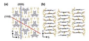
Fig. 2 Crystal structure of PCT-1·DMF: (a) Top view and (b) side view. The yellow molecules represent DMF. The gray, red, and purple atoms represent C, O, and N, respectively; H atoms are omitted for clarity.
