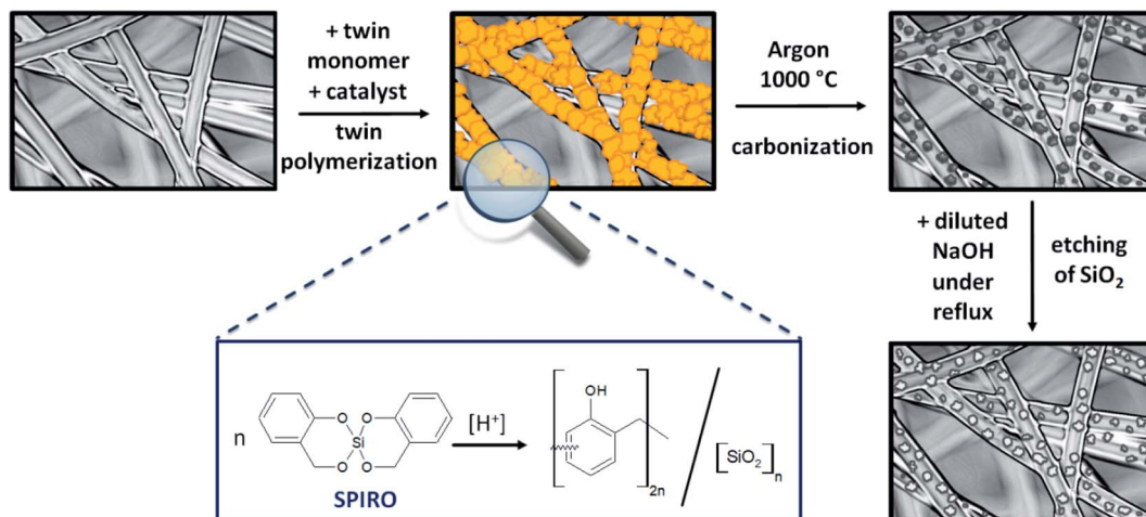
Fig. 1 Schematic illustration of the synthesis of porous C-C composite electrode material by coating a PAN-based felt substrate with hybrid material using the twin polymerization and subsequent pyrolysis and etching.
