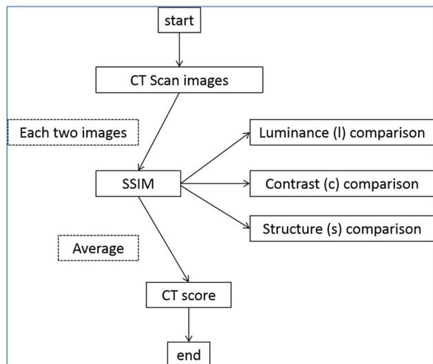
Fig. 3 CT score calculation flow chart. Each two CT images could get a CT score, the average of them are the output CT score of the tested battery.
