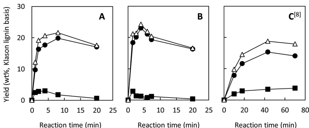
Fig. 1 Changes with time in yields of vanillin (●), vanillic acid (■), and their total yields (△) during degradation of Japanese cedar wood flour (14 mg) in 1.25 mol L<sup>-1</sup> Bu<sub>4</sub>NOH aq. (2.0 mL) under O<sub>2</sub> (A), under O<sub>2</sub> with the addition of NaOH(s) (200 mg) (B), and under air<sup>8</sup> (C) at 120 °C. The total amount of Klason lignin and acid-soluble lignin of the wood flour was 34.3 wt%.
