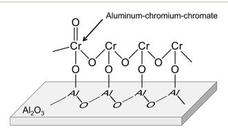
Fig. 10 Structure of aluminum-chromium-chromate.
