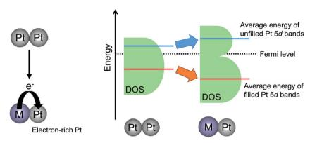
Fig. 6 Proposed effects of the promoters on the electronic state of Pt: (a) electron donation from the promoter (M) to Pt and (b) modification of the energy level of Pt 5d bands. Densities of states are denoted as DOS.
