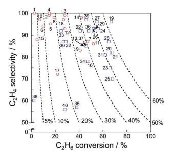
Fig. 11 Ethylene selectivity vs. ethane conversion of each catalyst presented in Tables 1 and 2. Dashed lines represent ethylene yield. Also, EDH in the absence and presence of  $CO_2$  are shown respectively with red circles and blue squares.
