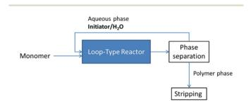
**Scheme 10** Simplified flow diagram of the process for the synthesis of silanol terminated PDMS *via* CROP.<sup>25</sup>
