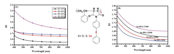
Fig. 2 (A) Refractive index curves of four polymers with different substituent elements at different wavelengths; (B) refractive index curves of six polymers with different monomer ratios at different wavelengths. Adapted with permission from ref. 35. Copyright 2019 The Royal Society of Chemistry.
