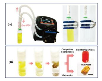
Fig. 11 (A) The equipment for simulating the dynamic extraction process in industrial treatment and the color change of the Au<sup>3+</sup> solution before and after treatment with the system; (B) procedure of gold extraction with Se-foam and posttreatments by competitive coordination or calcination. Reproduced with permission from ref. 216. Copyright 2020 WILEY-VCH Verlag GmbH & Co. KGaA, Weinheim.
