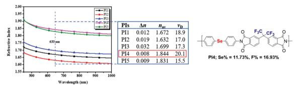
Fig. 1 Refractive index curves of five polyimide films and the structure of PI4. Adapted with permission from ref. 52. Copyright 2019 Elsevier Ltd.
