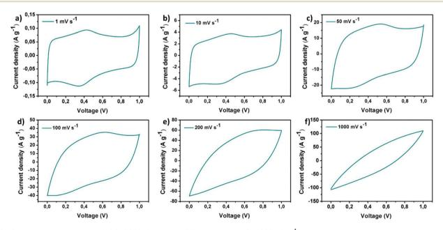
Cyclic voltammetry curves of rGO-POSS electrode at different scan rates  $(1-1000 \text{ mV s}^{-1})$ .
