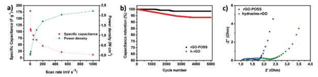
Fig. 5 (a) The dependence of specific capacitance and power density at various scan rates for rGO-POSS. (b) Cyclic stability of electrodes at  $100 \text{ mV s}^{-1}$  for rGO-POSS and h-rGO. (c) Comparison of Nyquist plots for rGO-POSS and hydrazine-reduced graphene oxide.
