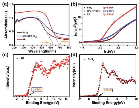
Fig. 8 (a) UV-vis diffuse reflection spectra, (b) Kubelka–Munk plots converted from the UV-vis diffuse reflection spectra, valence band spectrum of (c) RP and (d) SnS<sub>2</sub>.
