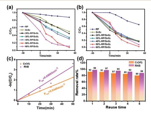
Fig. 2 Comparison of the effect of photocatalytic simultaneous removal of (a)  $Cr(v_1)$  and (b) RhB by RP, SnS<sub>2</sub>, and x-RP/SnS<sub>2</sub>, (c) the fitted reaction kinetic curves  $(-\ln(C/C_0) = kt)$  and (d) recycling test runs for five times in the photocatalytic removal of  $Cr(v_1)$  and RhB by 50%-RP/SnS<sub>2</sub>.
