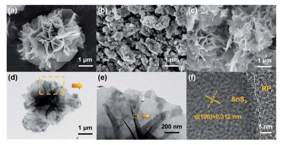
Fig. 3 SEM images of (a) SnS<sub>2</sub>, (b) RP, (c) 50%-RP/SnS<sub>2</sub>, (d and e) TEM and (f) HRTEM images of 50%-RP/SnS<sub>2</sub>
