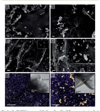
Fig. 1 (A–D) SEM images of  $MoS_{2(1-x)}Se_{2x}/N$ -rGO prepared using 6  $\mu l$ of DMDSe: (A) ATM precursor - 15 h at 200 °C without steptemperature heating; (B) ATM - 10 h at 180 °C + 5 h 200 °C; (C) ATM -15 h at 180 °C + 5 h 200 °C (inset: detail of  $MoS_{2(1-x)}Se_{2x}$  slab); (D)  $MoCl_5$  as Mo source – 15 h at 180 °C + 5 h 200 °C. (E and F) TEM of the sample shown in panel (C), before (E) and after annealing at 600 °C (F) (scale bar: 200 nm)
