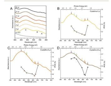
Fig. 6 (A) UV-Vis spectra of crystalline MoS $_{2(1-x)}$ Se $_{2x}$ /N-rGO crystalline samples. (B–D) IPCE measurements recorded at  $\eta=180$  mV for 0  $\mu$ l (B), 6  $\mu$ l (C) and 24  $\mu$ l (D) samples. In the plots, both the ICPE values (right axis) and the absorbance spectrum (left axis) of the sample are shown.
