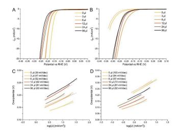
Fig. 4 Linear sweeps voltammetries for as-prepared (A) and crystalline (B)  $MoS_{2(1-x)}Se_{2x}/N$ -rGO samples. The related Tafel plots are reported for as-prepared (C) and crystalline (D) samples.
