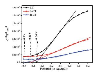
Fig. 6 Mott-Schottky plot of CT, S-CT and B-CT.
