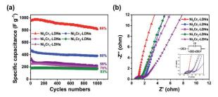
Fig. 6 (a) Cycle stability of LDN and LDH electrodes at 10 A  $\rm g^{-1}$ , and (b) Nyquist plots of LDN and LDH electrodes.
