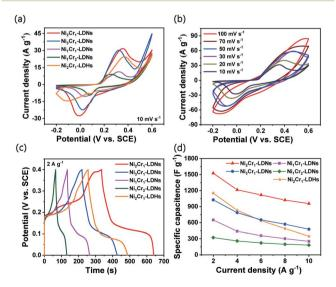
Fig. 5 (a) CV curves of LDN and LDH electrodes at a scan rate of 10 mV s $^{-1}$ , (b) CV curves of Ni<sub>2</sub>Cr<sub>1</sub>-LDNs at various scan rates from 5 to 100 mV s $^{-1}$ , (c) GCD curves of LDNs and LDHs at a current density of 2 A g $^{-1}$ , and (d) specific capacitances of LDN and LDH electrodes at different current densities.
