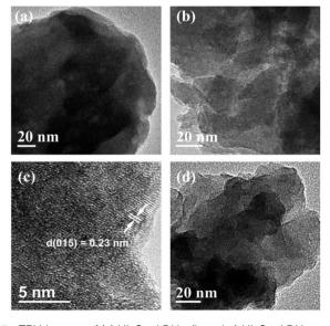
Fig. 3 TEM images of (a) Ni<sub>2</sub>Cr<sub>1</sub>-LDHs, (b and c) Ni<sub>2</sub>Cr<sub>1</sub>-LDNs and (d) Ni<sub>3</sub>Cr<sub>1</sub>-LDNs.
