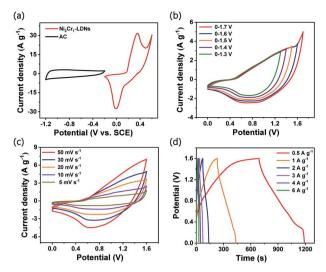
Fig. 7 (a) CV curves of  $\rm Ni_2Cr_1$ -LDNs and AC at a scan rate of 10 mV s<sup>-1</sup>, (b) CV curves of the ASC performed in different potential windows at 20 mV s<sup>-1</sup>, (c) CV curves at different scan rates from 5 to 50 mV s<sup>-1</sup>, and (d) GCD curves at different current densities.
