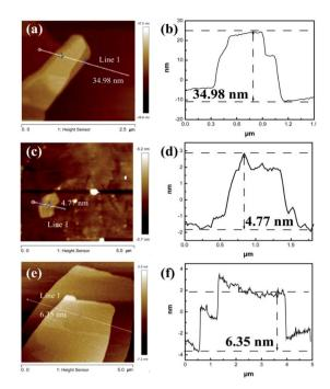
Fig. 2 AFM images and height profile of (a and b) Ni<sub>2</sub>Cr<sub>1</sub>-LDHs, (c and d) Ni<sub>2</sub>Cr<sub>1</sub>-LDNs, and (e and f) Ni<sub>3</sub>Cr<sub>1</sub>-LDNs.
