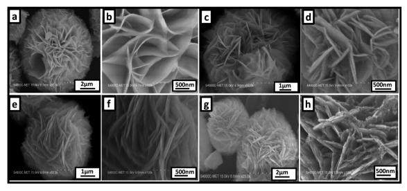
Fig. 2 Representative FE-SEM images of (a and b) pure  $Znln_2S_4$ , (c and d) 1%  $SnS@Znln_2S_4$ , (e and f) 2%  $SnS@Znln_2S_4$  and (g and h) 3%  $SnS@Znln_2S_4$  sample photocatalysts.
