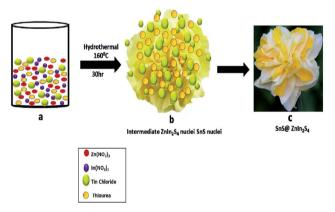
Scheme 1 Schematic of the formation mechanism of SnS@ZnIn<sub>2</sub>S<sub>4</sub> nano-heterostructures
