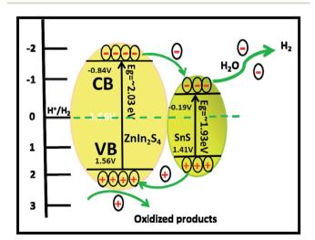
Scheme 2 Schematic of the photocatalytic mechanism of  $SnS@ZnIn_2S_4$  heterostructures.
