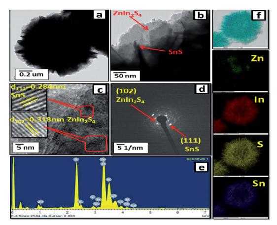
FE-TEM images (a and b), (c) HRTEM image, (d) SAED pattern, (e) EDAX spectra and (f) elemental mapping of 2% SnS-loaded ZnIn<sub>2</sub>S<sub>4</sub>.
