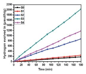
Fig. 7 Time versus volume of  $H_2$  (µmol  $h^{-1}$   $g^{-1}$ ) evolution from  $H_2O$  of all the samples synthesized at 160 °C for 30 h: (S0) pure SnS, (S1) pure Znln<sub>2</sub>S<sub>4</sub> and SnS@Znln<sub>2</sub>S<sub>4</sub> nano-heterostructures prepared with different percentages of SnS loading: (S2) 1%, (S3) 2% and (S4) 3%.
