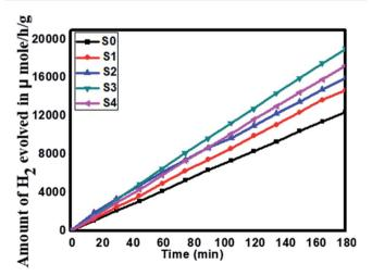
Fig. 8 Time versus volume of  $H_2$  (µmol  $h^{-1}$   $g^{-1}$ ) evolution from  $H_2S$  of all the samples synthesized at  $160\,^{\circ}C$  for 30 h: (S0) pure SnS, (S1) pure ZnIn<sub>2</sub>S<sub>4</sub> and SnS@ZnIn<sub>2</sub>S<sub>4</sub> nano-heterostructures prepared with different percentages of SnS loading: (S2) 1%, (S3) 2%, and (S4) 3%.
