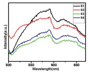
Fig. 5 UV-DRS spectra of (S1) pure  $Znln_2S_4$ , (S2) 1%  $SnS@Znln_2S_4$ , (S3) 2%  $SnS@Znln_2S_4$  and (S4) 3%  $SnS@Znln_2S_4$  sample photocatalysts.
