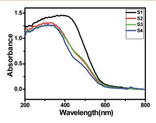
Fig. 4 UV-DRS spectra of (S1) pure  $ZnIn_2S_4$ , (S2) 1%  $SnS@ZnIn_2S_4$ , (S3) 2%  $SnS@ZnIn_2S_4$  and (S4) 3%  $SnS@ZnIn_2S_4$  sample photocatalysts.
