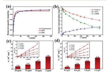
Fig. 6 Kinetics analysis of  $\gamma$ -Fe<sub>2</sub>O<sub>3</sub>@PANI@TiO<sub>2</sub>: (a) adsorption kinetics in the dark, (b) reaction kinetics of As(III) and As(V) under a Xe lamp, (c) the reaction rate constants and fitting curves (inset) at various initial As(III) concentrations, and (d) the reaction rate constants and fitting curves (inset) at various concentrations of the catalyst.
