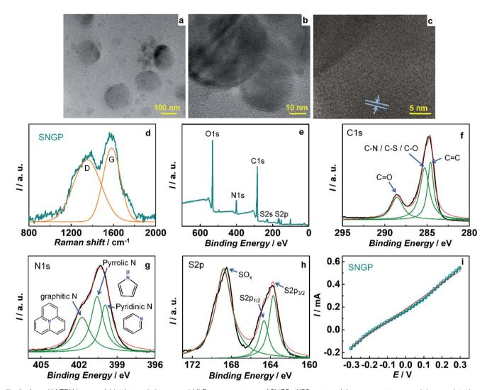
Fig. 2 (a and b) TEM images, (c) lattice scale image and (d) Raman spectrum of SNGPs. XPS spectra: (e) survey spectrum, and deconvoluted core level spectra for (f) C1s, (g) N1s and (h) S2p of SNGPs. (i) I-V characteristics of SNGPs.
