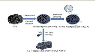
Fig. 1 The schematic of the preparation process of N, O-PC-CNTs, N, O-PC and PC.
