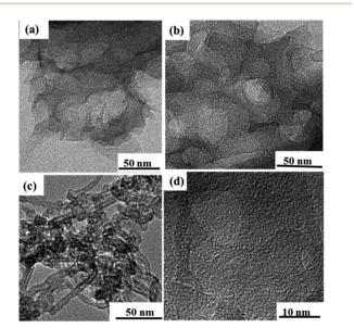
Fig. 3 TEM images of as prepared samples (a) PC, (b) N, O-PC, (c) N, O-PC-CNTs samples, and (d) the HRTEM image of N, O-PC-CNTs samples.
