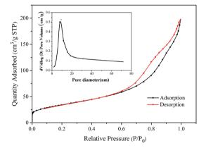
Fig. 4 Nitrogen adsorption–desorption isotherms and pore size distribution curve of  $Ni-TiO_2$ .
