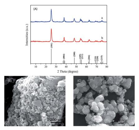
Fig. 2 (A) XRD patterns of (a) TiO<sub>2</sub> and (b) Ni-TiO<sub>2</sub> nanoparticles; (B) morphology of Ni-TiO<sub>2</sub>; (C) morphology of TiO<sub>2</sub>.
