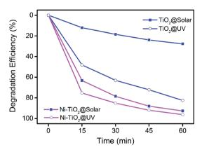
Fig. 5 Photodegradation of MB dye using TiO<sub>2</sub> and Ni-TiO<sub>2</sub> nanoparticles under UV and solar light irradiation.
