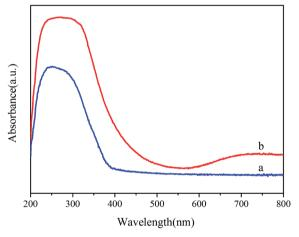
Fig. 3 UV-visible absorption spectra of (a)  ${\rm TiO_2}$  and (b)  ${\rm Ni-TiO_2}$  samples.
