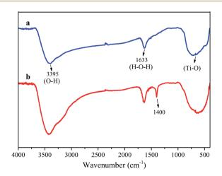
Fig. 1 FT-IR spectral analysis of (a) TiO<sub>2</sub> and (b) Ni-TiO<sub>2</sub> nanoparticles.
