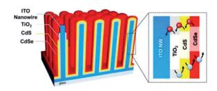
Fig. 6 Schematic illustration of the CdSe/CdS/TiO<sub>2</sub>/ITO multi-shell photoanode. Reproduced with permission from ref. 77; Copyright (2016) American Chemical Society.
