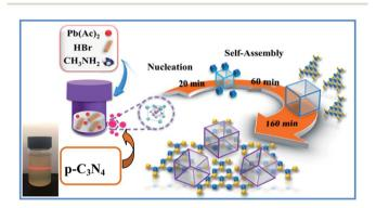
Fig. 1 Schematic illustration of the formation and morphological evolution process of MAPbBr<sub>3</sub>/p-g-C<sub>3</sub>N<sub>4</sub> composites using a p-g-C<sub>3</sub>N<sub>4</sub> sol solution through a solvothermal method.
