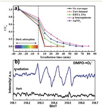
Fig. 7 (a) Effect of radical scavenger/quencher including p-benzoquinone (p-BQ), ethylenediaminetetraacetic acid disodium salt (EDTA-2Na), tert-butanol (t-BuOH) and AgNO<sub>3</sub> on the degradation process of MG. (b) ESR spectra of the MAPbBr<sub>3</sub>/p-g- $C_3N_4$ -1.0 mg sample without and with visible-light irradiation for 5 min for the detection of 'O2' radicals.
