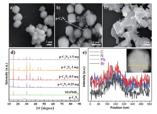
Fig. 2 (a-c) SEM images of MAPbBr $_3$ /p-C $_3$ N $_4$ -0, -1.0, and -1.5 mg samples, respectively. (d and e) The corresponding XRD patterns and EDS line scan image of an individual MAPbBr<sub>3</sub> microcrystal encapsulated nanosheet.
