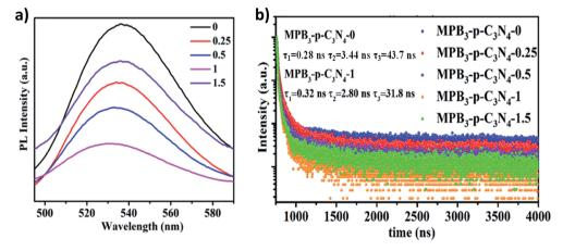
Fig. 8 (a) Steady-state PL spectra and (b) time-resolved photoluminescence decay spectra (TRPL) of MAPbBr<sub>3</sub>/p-g-C<sub>3</sub>N<sub>4</sub> (loading amount: 0-1.5 mg) samples.
