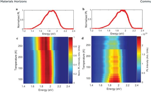
Fig. 4 Normalized photoluminescence spectrum at (a) room temperature, (b) 150 K, (c) normalized as a function of temperature, and (d) as a function of temperature without intensity normalization. Excitation at 2.95 eV.
