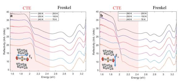
Fig. 2 Temperature dependence of the near-normal-incidence reflectivity spectra of perylene—TBPA with light polarized (a) parallel and (b) perpendicular to the TBPA long axis. Spectra are offset for clarity. The graph is divided into two regions, denoting the excitation of Frenkel excitons (white area) and CTEs (pink shaded area). Insets show the polarization of light in relation to the TBPA long axis and crystal structure simplified here with a trimer.
