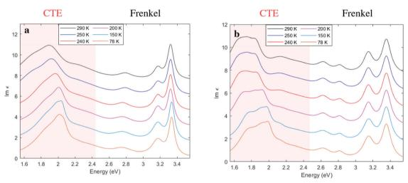
Fig. 3 Temperature dependence of the imaginary part of the dielectric function – which is proportional to light absorption – of perylene–TBPA with light polarized (a) parallel and (b) perpendicular to the TBPA long axis. Spectra are offset for clarity.
