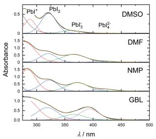
Fig. 3 (a) Absorbance spectra of MAPbI<sub>3</sub> solutions in DMSO, DMF, NMP, and GBL.
