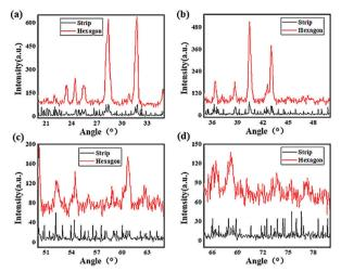
**Fig. 5** XRD spectral analysis of different  $CH_3NH_3Pbl_3$  perovskites. (a) Diffraction angle range from 20° to 35°; (b) diffraction angle range from 35° to 50°; (c) diffraction angle range from 50° to 65°; and (d) diffraction angle range from 65° to 80°.
