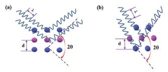
Fig. 6 Schematic illustration of XRD for the structural transformation of the CH<sub>3</sub>NH<sub>3</sub>PbI<sub>3</sub> perovskite.
