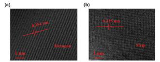
Fig. 3 (a and b) Lattice fringes of different  $CH_3NH_3PbI_3$  perovskite crystals characterized by TEM.
