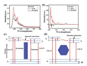
Fig. 7 (a) Emission spectra of different shaped CH<sub>3</sub>NH<sub>3</sub>PbI<sub>3</sub> perovskites; (b) excitation spectra of different shaped CH<sub>3</sub>NH<sub>3</sub>Pbl<sub>3</sub> perovskites; and (c and d) schematic illustration of the fluorescence mechanisms for different shaped CH<sub>3</sub>NH<sub>3</sub>Pbl<sub>3</sub> perovskites
