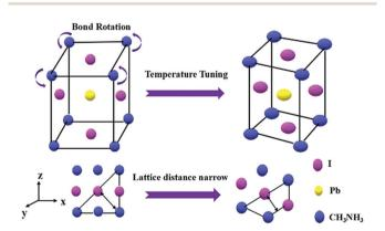
Fig. 4 Schematic illustration of the structural transformation of the  $CH_3NH_3PbI_3$  perovskite.
