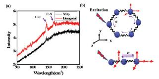
Fig. 8 (a) Raman spectra of different shaped CH<sub>3</sub>NH<sub>3</sub>Pbl<sub>3</sub> perovskites and (b) schematic illustration of the Raman scattering for different shaped CH<sub>3</sub>NH<sub>3</sub>Pbl<sub>3</sub> perovskites.
