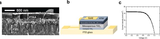
Fig. 6 (a) Cross section SEM image of the PSC with a ratio of 80: 20 (CsSn<sub>0.2</sub>Pb<sub>0.8</sub>I<sub>2.6</sub>Br<sub>0.4</sub>) (Pb: Sn) and PTAA as the HTM. (b) Schematic illustration of the perovskite solar cell configuration used in this work. (c) JV curve of the champion cell presenting 12.7% efficiency, a FF of 64.2%, a  $J_{sc}$  of 19.09 mA cm<sup>-2</sup> and a  $V_{oc}$  of 1 V.
