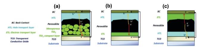
Fig. 1 Perovskite solar cell architectures: (a) n-type  $TiO_2$  mesoporous-based; (b) planar "n-i-p"; (c) planar "p-i-n". Illumination occurs from the substrate side. In all these cases, the substrate can be either a glass or polymer foil. Reproduced with permission from ref. 48. Copyright © 2017 The Royal Society of Chemistry.
