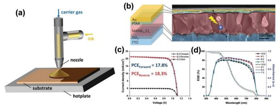
Fig. 6 Spray coating. (a) Schematic of the spray coating process. (b) SEM cross-sectional image of a high-quality spray-coated MAPbI $_{3-x}$ Cl $_x$  perovskite absorber. (c) PCEs up to 18.3% in reverse J-V characteristics and (d) high external quantum efficiency (EQE) were achieved, which is a result of a careful solvent engineering of the spray process. Reproduced with permission from ref. 91. Copyright © 2019 WILEY-VCH.
