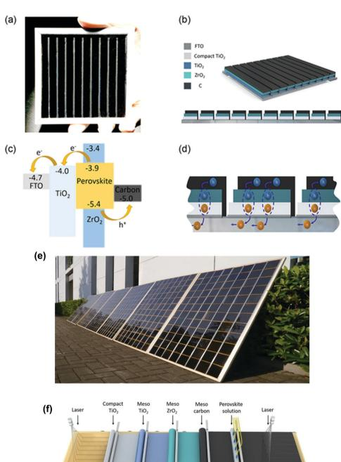
Fig. 7 (a) Image of a monolithic printable PSM with 10 subcells. (b) The monolithic interconnection scheme of the module. (c) Energy level diagrams of the hole-conductor-free printable PSC. (d) Schematic of the electron and hole separation on a serially connected PSM. (e) Image of 7 m<sup>2</sup> printable perovskite solar panels. (f) Schematic of the proposed production line of PSMs. Reproduced with permission from ref. 98. Copyright ( 2017 WILEY-VCH.
