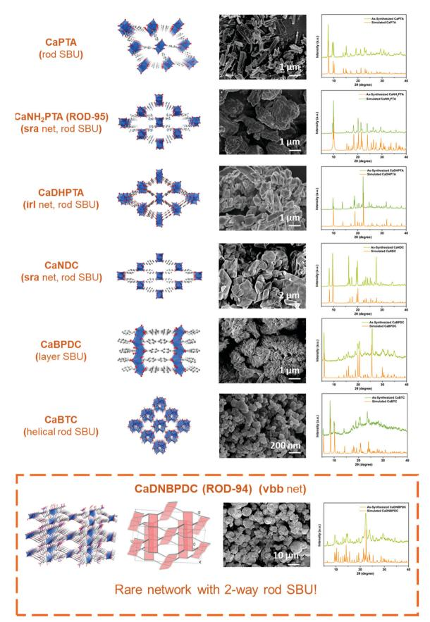
Fig. 2 The seven selected rod/layer MOFs synthesized by the room-temperature fast scale-up synthesis method. Crystal structures, SEM images, and PXRD patterns are shown in rows. The structure of newly synthesized CaDNBPDC (ROD-94) with an unusual underlying net is highlighted in the red dashed box.
