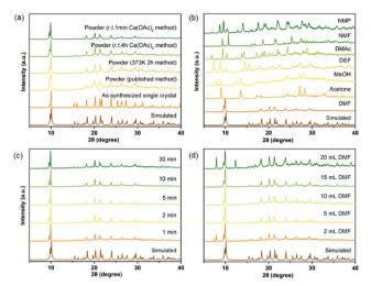
Fig. 1 Optimization of reaction conditions for CaNH<sub>2</sub>PTA (ROD-95) indicated by phase purity: (a) synthetic method, (b) types of organic solvents, (c) reaction time and (d) amount of DMF.
