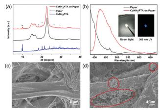
Fig. 5 Preparation of the luminescent test paper: (a) PXRD patterns of the as-made paper loaded with CaNH $_2$ PTA (ROD-95; asterisks represent the peaks of MOF); (b) emission spectra of fluorescent and bare paper (insets show the test paper under room light and 365 nm UV light) and (c and d) SEM images of the substrate without and with MOF loading (red circles indicate the growth of MOF particles on paper fibres).
