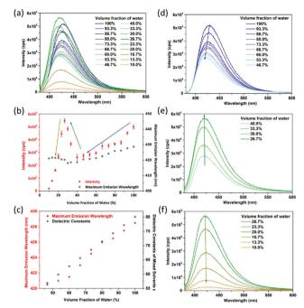
Fig. 4 Luminescence sensing of the water content in DMF through selfdisintegration of CaNH<sub>2</sub>PTA (ROD-95): (a) emission spectra with different water contents, (b) luminescence intensity and maximum emission wavelength as a function of water volume fraction, (c) the relationship between maximum emission wavelength and dielectric constants, and (d-f) emission spectra of the three segments.
