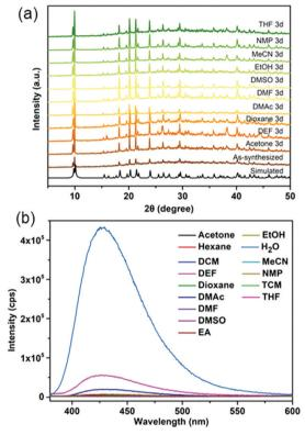
Fig. 3 (a) Solvent stability of CaNH<sub>2</sub>PTA (ROD-95) monitored using PXRD patterns after immersion for 3 days; (b) selective sensing of water monitored using the emission spectra of CaNH<sub>2</sub>PTA in supernatants of various solvents in 1 min.
