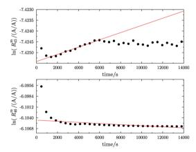
(c) Logarithms of  $R_{45}^{m}$  and  $R_{46}^{m}$  against time during the measurement of parent material A. Prior to the measurement, an aliquot of the gas was filled in one of the gas spheres. Previous to the filling with gas A, a platinum band was placed into the sphere. Subsequently, the sphere was heated for 39.5 h with a Bunsen burner ( $\theta \approx 1800\,^{\circ}\text{C}$ ).
