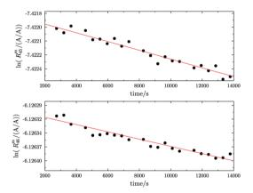
(b) Logarithms of  $R_{45}^{\rm m}$  and  $R_{46}^{\rm m}$  against time during the measurement of parent material A. Prior to the measurement, an aliquot of the gas was filled in one of the gas spheres and heated for 48 h with a Bunsen burner ( $\vartheta \approx 1800\,^{\circ}$ C). (Six outliers were removed.)
