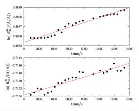
(b)  $\ln(R_{45}^m)$  against time (top) and  $\ln(R_{46}^m)$  against time of blend b2 (bottom). The blend was heated with a Bunsen burner for 11.8 h before the measurement. The red line in both graphs indicates a linear fit.
