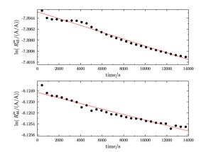
(a) Logarithms of  $R_{45}^{\rm m}$  (top) and  $R_{46}^{\rm m}$  (bottom) against time during the measurement of parent material A ( $^{12}$ C enriched material). The gas was heated prior to the measurement for 25 h with a Bunsen burner ( $\vartheta \approx 1800 \,^{\circ}$ C).
