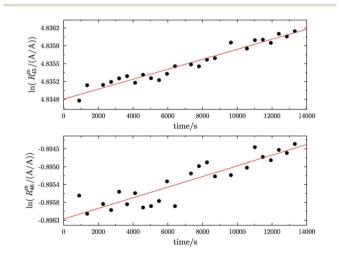
Fig. 8 Logarithms of  $R_{45}^{\rm m}$  (top) and  $R_{46}^{\rm m}$  (bottom) against time during the measurement of parent material B (13C enriched material). The gas was heated prior to the measurement for 13 h using a Bunsen burner ( $\vartheta$ ≈ 1800 °C).
