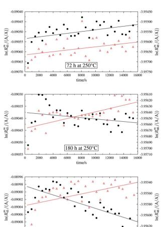
Fig. 2 Heating history of blend b1. Top:  $\ln(R_{45}^m)$  (black dots) and  $\ln(R_{46}^m)$  (red triangles) against time after heating at 250 °C for 72 h. Centre:  $\ln(R_{45}^m)$  and  $\ln(R_{46}^m)$  against time after heating at 250 °C for 180 h. Bottom:  $\ln(R_{45}^m)$  and  $\ln(R_{46}^m)$  against time after heating at 250 °C for 600 h. Mind the different scales.
