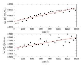
(a)  $\ln(R_{45}^m)$  against time (top) and  $\ln(R_{46}^m)$  against time of blend b2 (bottom). The blend was heated with a Bunsen burner for 5h before the measurement. The red line in both graphs indicates a linear fit.
