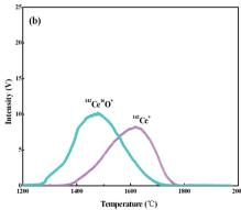
Fig. 2 Intensities of <sup>142</sup>Ce<sup>+</sup> and <sup>142</sup>Ce<sup>16</sup>O<sup>+</sup> as a function of the temperature: (a) FPIE filament; (b) traditional double Re filaments. Approximately 1 μq Ce was loaded on the filament, and the Faraday cup configuration is shown in Line 3 of Table 3.
