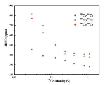
Fig. 4 External precisions (2RSD) of different Ce isotope ratios as a function of <sup>138</sup>Ce<sup>+</sup> beam intensity. The measurements were performed in Ce<sup>+</sup> mode with FPIE filaments loaded with 5 µg Ce.
