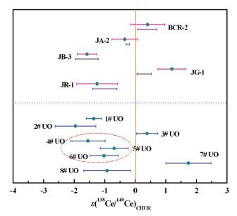
Fig. 6 The  $\varepsilon \mathrm{Ce}$  values of reference rock samples and uranium ore samples. The bars below the  $\varepsilon$ Ce values of reference rock samples represent the reported  $\varepsilon$ Ce values in Table 6, and the vertical line represents  $\varepsilon Ce = 0$ .
