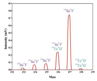
Fig. 3 The formation of BaF<sup>+</sup> ions at masses 153, 154, 155, 156 and 157 with FPIE filament (T=1200 °C).
