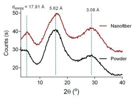
Fig. 5 Wide-angle XRD patterns of the 6FDA-TrMPD polymer and nanofihers
