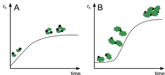
**Fig. 3** Measurable changes in hydrodynamic radius,  $r_H$ , as function of time for heteroaggregation of ENPs (black circles) and SPM (green clouds). A: ENPs and SPM of similar size. B: SPM orders of magnitude larger than ENPs.
