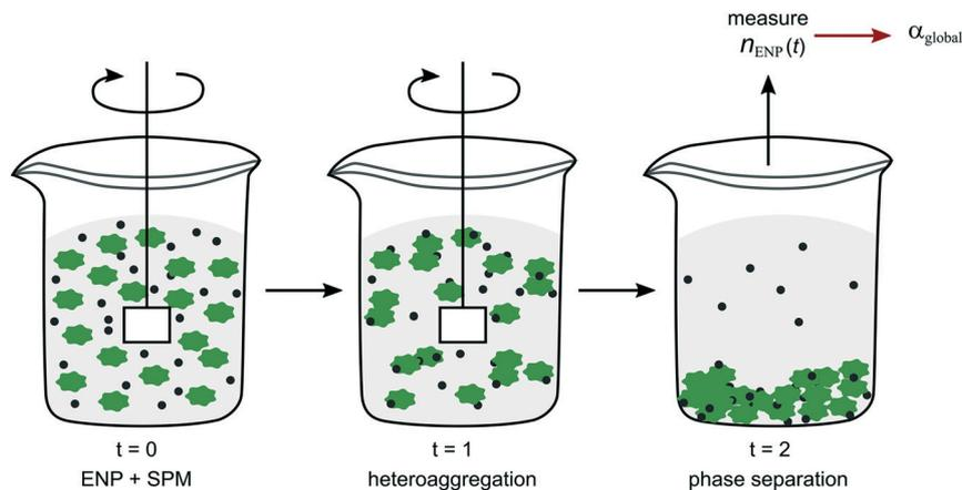
Fig. 5 Schematic representation of the experimental set-up of the batch method as described in Barton *et al.*<sup>77</sup> and Geitner *et al.*<sup>78,79</sup>
