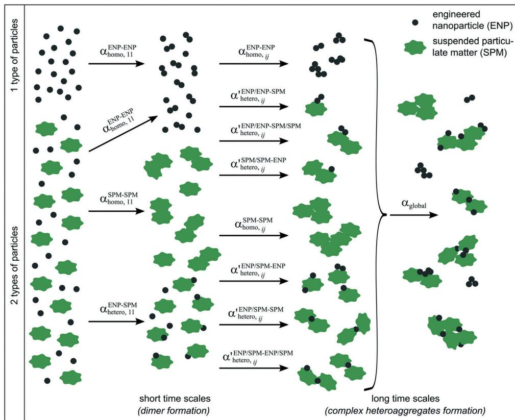
**Fig. 2** Schematic representation of increased complexity of possible homo- and heteroaggregation pathways with the corresponding  $\alpha$  values in a system containing two types of particles versus one particle type.
