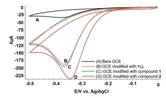
Fig. 6 Voltammetric response of (A) bare GC electrode; (B) GC electrode modified with  $H_2L$ , (C) GC electrode modified with compound 1, and (D) GC electrode modified with compound 2 in 1.4 mM  $H_2O_2$ .
