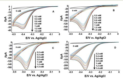
Fig. 5 Electrochemical reduction of  $H_2O_2$  (various concentrations) on (A) bare GC electrode, (B) GC electrode modified with  $H_2L$ , (C) GC electrode modified with compound 1, and (D) GC electrode modified with compound 2.
