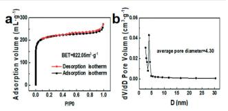
**Fig. 3** Nitrogen adsorption–desorption isotherms (a) and corresponding pore size distribution (b) of NC@Ru-3.
