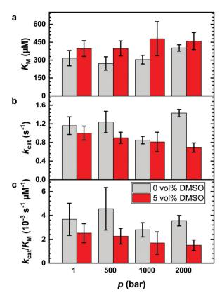
Fig. 4 Pressure dependence of the kinetic parameters for the hydrolysis of the substrate AAF-AMC catalyzed by the enzyme  $\alpha\text{-CT}$  at 20  $^{\circ}\text{C}$  in neat buffer (grey bars) and in the presence of 5 vol% DMSO (red bars). (a) Michaelis constant,  $K_{M}$ , (b) turnover number,  $k_{cat}$ , and (c) catalytic efficiency,  $k_{cat}/K_{M}$ .
