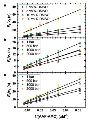
Fig. 1 Lineweaver-Burk plots for the hydrolysis of AAF-AMC catalyzed by the enzyme  $\alpha$ -CT. (a) Plots at ambient pressure as function of DMSO vol%: neat buffer (blue); 5 vol% DMSO (red); 10 vol% DMSO (green); 20 vol% DMSO (orange). (b) Plots in neat buffer at different pressures: 1 bar (blue); 500 bar (red); 1000 bar (green); 2000 bar (orange). (c) Plots in buffer containing 5 vol% DMSO at different pressures: 1 bar (blue); 500 bar (red); 1000 bar (green); 2000 bar (orange)
