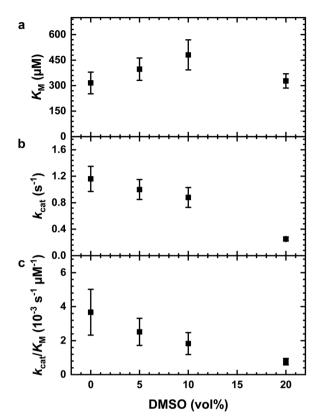
Fig. 2 Effect of DMSO (in vol%) on the kinetic parameters for the hydrolysis of AAF-AMC catalyzed by the enzyme lpha-CT. (a) Michaelis constant,  $K_{\rm M}$ , (b) turnover number,  $k_{\rm cat}$ , and (c) catalytic efficiency,  $k_{\rm cat}/K_{\rm M}$ . Buffer conditions: 0.1 M Tris, 10 mM CaCl<sub>2</sub>, pH 7.8; T = 20 °C, p = 1 bar.
