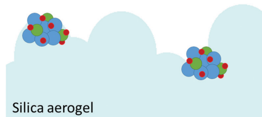
Fig. 12 Schematic of the CoRe-gel in 5% ammonia at 600 °C with the major species consisting of rhenium (blue), cobalt (green) and oxygen/nitrogen (red).
