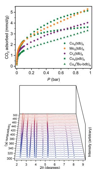
Fig. 3 (Top)  $CO_2$  adsorption in  $M_4(L)_4$  cages at 195 K. (Bottom) PXRD patterns as a function of temperature for  $Cu_4(tdb)_4$  spanning the temperature range of 300-550 K. During this activation, the cage remains moderately crystalline while undergoing significant structural rearrangement.
