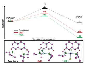
Fig. 3 DFT calculated (BP86-D3, def2-TZVP) free energy profiles ( $\Delta G_{298K}^0$ in kcal mol<sup>-1</sup>) for the rearrangement of **PONNOP** to **PONNP** (top) and the transition state geometries (bottom).
