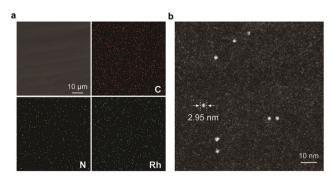
Fig. 2 (a) Top view of the SEM image and EDX mapping of ElastoMOP-3. (b) HAADF-STEM image of ElastoMOP-3.
