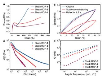
Fig. 3 (a) Tensile stress-strain curves of the ElastoMOPs 1-3. Deformation rate:  $100 \text{ mm min}^{-1}$ . (b) Cyclic stress-strain tests of ElastoMOP-3. Deformation rate: 100 mm min<sup>-1</sup>. (c) Step-strain (10%) relaxation curves of ElastoMOPs **1-3** at 40 °C. (d) Frequency sweeps from oscillatory rheometry of ElastoMOPs 1-3 at a 5.0% strain amplitude
