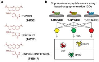
Fig. 1 (a) Structure of the 5-TAMRA-labeled peptide probes T-RS5, T-QY7 and T-ED17. (b) Schematic illustration of the supramolecular fluorogenic peptide sensor array based on graphene oxide (GO) for differential sensing of three viruses including ebola virus (EBOV), marburg virus (MARV) and receptor-extensive vesicular stomatitis virus (VSV) using the principal component analysis (PCA).
