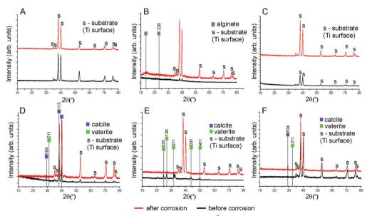
Fig. 6 X-ray diffractograms of the bare Ti surface (A); Ti surface coated with Ca<sup>2+</sup>-crosslinked Alg hydrogel (Ti-Alg) (B); Ti surface coated with dextran sulfate (Ti-DS) (C); Ti surface mineralized with CaCO<sub>3</sub> (Ti-CaCO<sub>3</sub>) (D); Ti surface coated with CaCO<sub>3</sub>-mineralized Ca<sup>2+</sup>-crosslinked Alg hydrogel (Ti-Alg-CaCO<sub>3</sub>) (E); and Ti surface coated with CaCO<sub>3</sub>-mineralized dextran sulfate (Ti-DS-CaCO<sub>3</sub>) (F).
