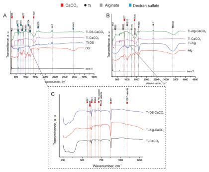
Fig. 4 ATR-FTIR spectra of the bare Ti surface and Ti surfaces with modifications: (A) spectra of Ti-DS, Ti-DS-CaCO $_3$ , Ti-CaCO $_3$  and dextran sulfate powder; (B) spectra of Ti-Alg, Ti-Alg-CaCO $_3$ , Ti-CaCO $_3$  and Ca<sup>2+</sup>-crosslinked Alg hydrogel; and (C) spectra of mineralized Ti surfaces (Ti-CaCO $_3$ , Ti-Alg-CaCO $_3$ , Ti-DS-CaCO $_3$ ) in the wavenumber range 250–1300 cm<sup>-1</sup>.
