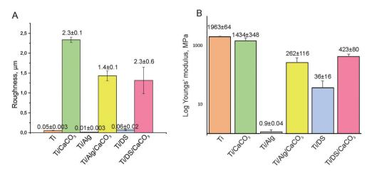
Fig. 7 Average surface roughness of the modified Ti surfaces (A); the average Youngs' modulus of the modified Ti surfaces (B).
