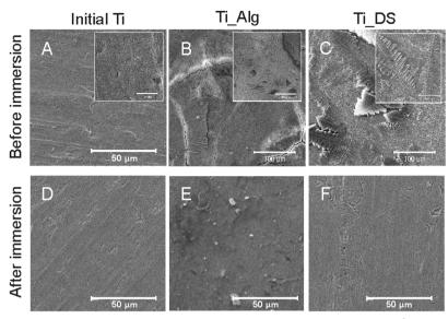
Fig. 1 SEM images of the bare Ti surface before (A) and after the corrosion process (D); Ti plate coated with Ca<sup>2+</sup>-crosslinked alginate hydrogel (Ti-Alq) before (B) and after the corrosion process (E); and Ti surface coated with dextran sulfate (Ti-DS) before (C) and after the electrochemical tests (F). The scale segment of the magnified image insets in the upper row is 10 µm.
