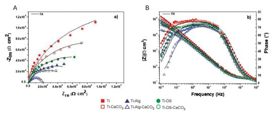
Fig. 8 Nyquist (A) and Bode (B) phase and amplitude plots of the impedance data (scattered points – measured impedance data, solid line – fitted curves).
