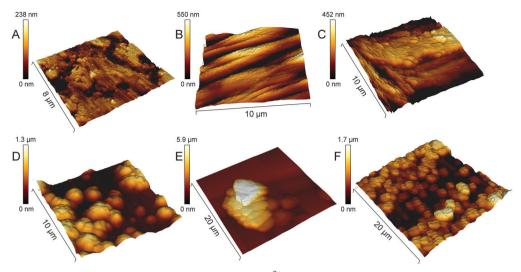
Fig. 5 AFM topography of Ti surfaces: unmodified (A), and coated with Ca<sup>2+</sup>-crosslinked Alg hydrogel (Ti-Alg) (B); Ti surface coated with dextran sulfate (Ti-DS) (C); Ti surface mineralized with CaCO<sub>3</sub> (Ti-CaCO<sub>3</sub>) (D); Ti surface coated with CaCO<sub>3</sub>-mineralized Ca<sup>2+</sup>-crosslinked Alg hydrogel (Ti-Alg-CaCO<sub>3</sub>); (E); and Ti surface coated with CaCO<sub>3</sub>-mineralized dextran sulfate (Ti-DS-CaCO<sub>3</sub>) (F).
