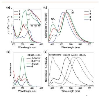
Fig. 4 (a) UV-vis absorption spectra of 1–4 in toluene ( $10^{-5}$  M). The inset shows a magnified view of the lower-energy ICT absorption bands. (b) Theoretical absorption spectra of 1–4 with different populations of QE/QA conformers simulated using TD-DFT (LC- $\omega$ PBE/6-31+G(d)). (c) Steady-state PL spectra of 1–4 in the deoxygenated toluene solutions. (d) Solvatochromic PL responses of 1 in different solvents upon excitation at 350 nm.
