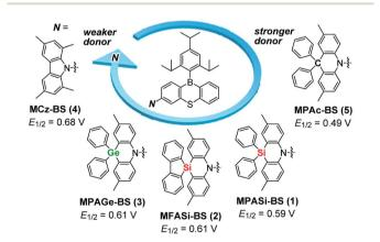
Fig. 1 Molecular structures of blue phenothiaborin-based TADF emitters incorporating acridan-analogous donors with different group 14 elements.  $E_{1/2}$  values represent the half-wave oxidation potentials vs. Fc/Fc<sup>+</sup> determined by cyclic voltammetry and differential pulse voltammetry (ESI†), as a measure of the electron-donating ability.
