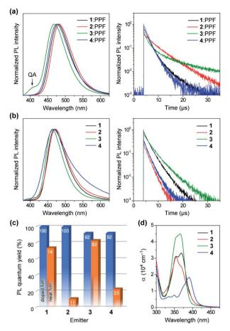
Fig. 6 (a and b) Steady-state PL spectra (left) and transient PL decay profiles (right) of 1-4 in (a) 50 wt%-emitter:PPF doped films and (b) pure neat films measured at 300 K under  $N_2$ . (c) Comparison of  $\Phi_{Pl}$ values measured with 1-4 in the doped and neat films. (d) UV-vis absorption spectra of the neat films of 1-4.
