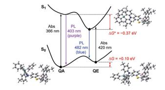
Fig. 5 Schematic energy level diagram for 3 exhibiting the mechanism of excited-state interconversion and dual PL emissions in toluene solution. The optimized structures of the QA and QE conformations in the  $S_0$  state and the orthogonal conformation in the  $S_1$  state calculated at the B3LYP/6-31G(d) level are presented.
